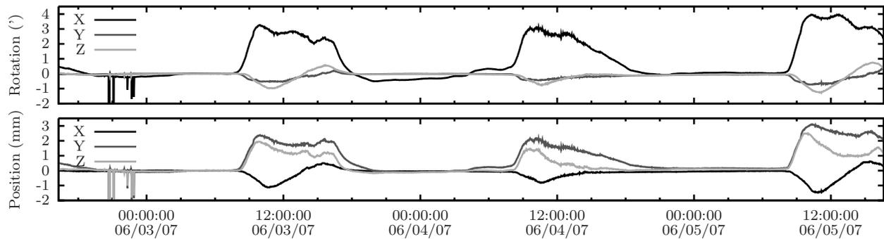
**Figure 5.** The difference in the motion between the primary and secondary mirrors as measured by the fiducial points over three days. The  $(x, y, z)$  coordinate system is described in Fig. 4. On these dates, sunrise was at about 7:05 and sunset at 17:50. The structure is most unstable between these times. *Top:* The differences in rotation about the three axes. *Bottom:* The differences in position.
