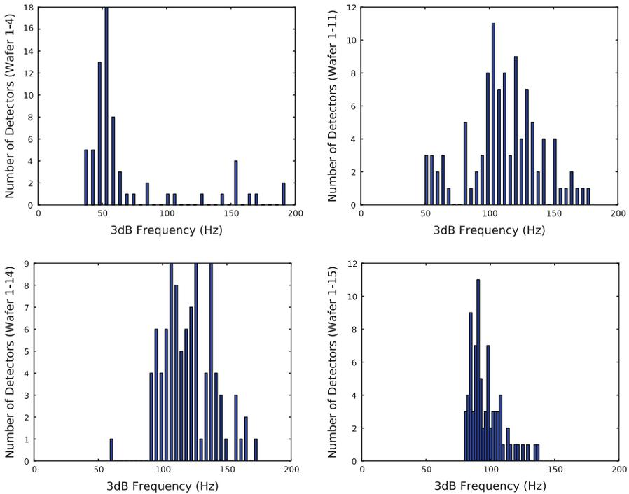
**Fig. 3** Above are distributions of 3dB frequencies for the four wafers and for individual detectors in the ABS focal plane. Note that there are 18 detectors with 3dB frequencies above 200 Hz, but the frequency scale has been truncated at 200 Hz for clarity. (Color figure online)
