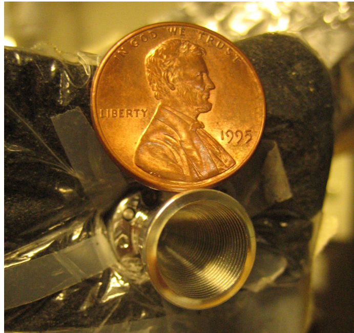
Figure 2.15: Photo of an ABS feedhorn with a penny for scale. The corrugations are partially visible.
