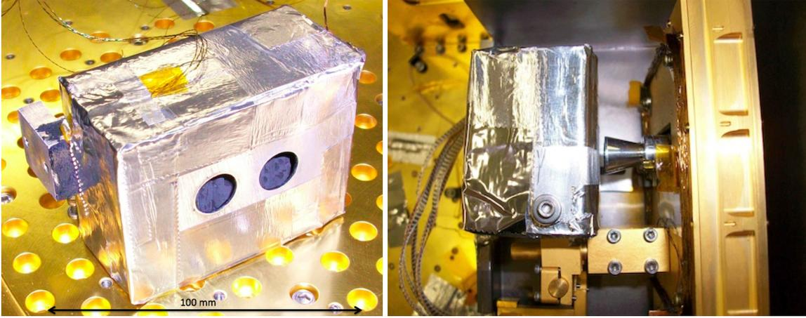
Figure 2. (Left) The cold load before installation resting on the 4 K plate. The eccosorb is visible through feedhorn holes in the Al 1100 radiation shield. (Right) The load installed in front of horns, which are later partially inserted within the load shield. Each horn is attached to an individual pixel mounted inside a gold-plated copper box thermally sunk to the mK stage.
