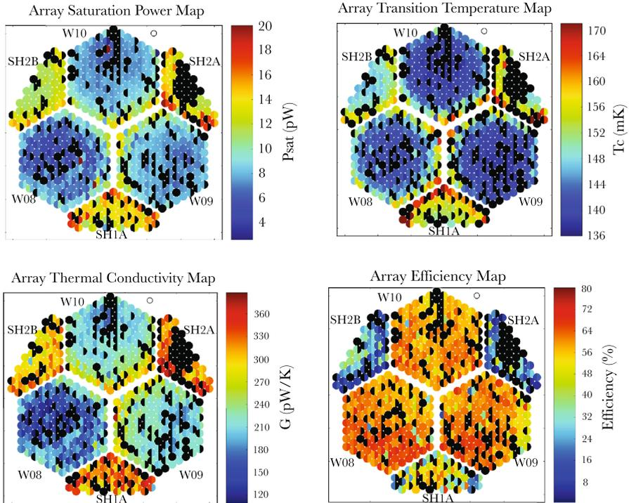
**Fig. 1** Maps of measured detector parameters across the array. *Black regions* indicate non-functioning detectors or detectors that are not read out. The parameters are fairly uniform on the wafer level, with the largest differences occurring among wafers. Variation on the wafer occurs in a radial pattern with slightly elevated  $P_{\text{sat}}$ ,  $T_c$ , and  $G$  values at the very edges of the wafers (Color figure online)
