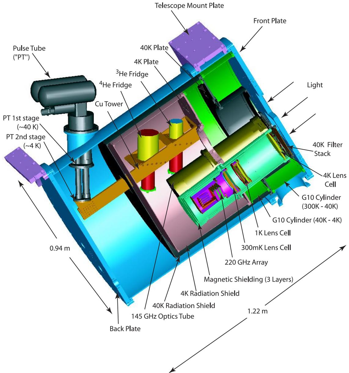
Figure 1. Cut away of the MBAC cryostat showing the location of the internal components. A cut away of the 220 GHz optics tube is also shown, giving the location of its lenses, filters, and array, which is similar for all three tubes. The 280 GHz optics tube mounts just above the 145 and 220 GHz optics tubes, but is removed for clarity. The connection of the first stage of the pulse tube and its radiation shielding to the 40K plate is also omitted for clarity.
