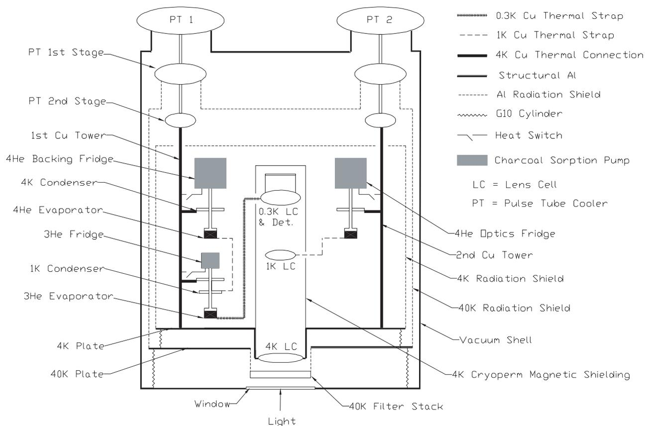
Figure 5. Schematic of the radiation shielding and thermal connections in the MBAC. Only a single optics tube is shown, but all are connected in a similar way and in parallel.
