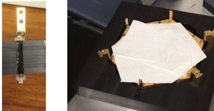
Figure 8. Screws stack silicon wafer together (left, photo courtesy to Shuay-Pwu Ho). To protect the silicon wafers, two Teflon washers are used for each screw, separating the wafer stack and metal part. The Delrin jig helps to align the L-brackets orientations (right). It is designed so that the top surface of the feedhorn stack is at the same level as the top surface of the jig.
