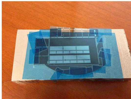
Figure 2. A silicon rectangular template that has outlines for mux and interface chips is taped down to a metal base with blue low-tack tape. The surrounding four silicon pieces are also taped down, so that later when replacing the template with a real wiring chip, the wiring chip will sit on the metal base in exactly the same position as the template.
