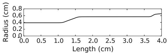
**Fig. 6** The profile of the AdvACT LF spline-profiled feedhorn is shown. The total length of the feedhorn is 4 cm. Spline-profiled horns exhibit good beam symmetry and beam coupling efficiency for their compact size
