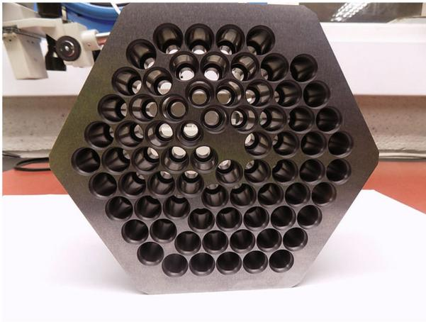
**Fig. 7** The full LF AdvACT feedhorn array prior to gold coating. The array is direct machined out of a Si–Al alloy (Color figure online)
