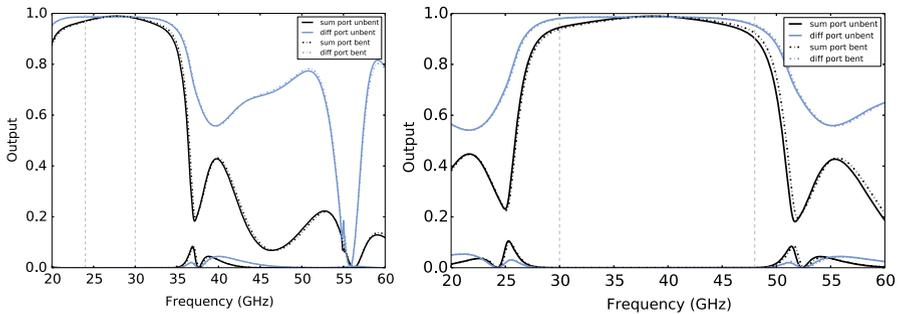
**Fig. 4** The sum (black) and difference (light blue) port responses of the hybrid tee are shown for the 27 GHz (left) and 39 GHz (right) bands. The solid lines are the unbent hybrid responses, while the dashed lines show the bent hybrid responses. The change is negligible (Color figure online)
