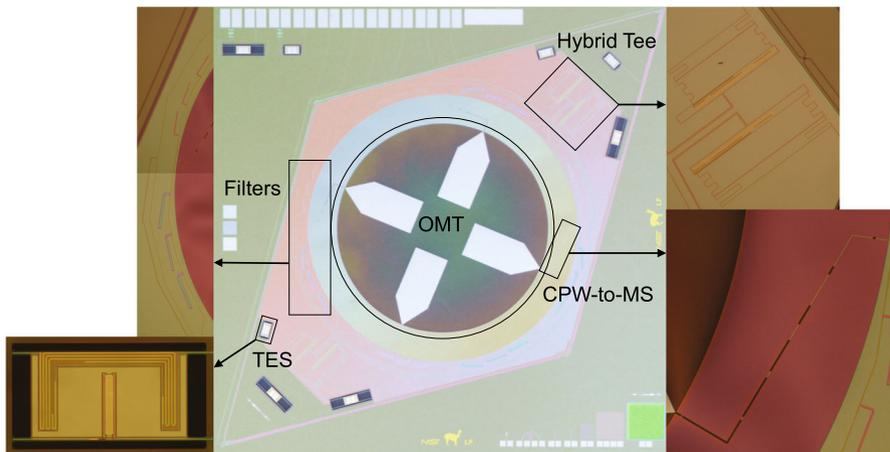
**Fig. 1** A prototype LF pixel is shown. Light is coupled through the 7.8-mm-diameter OMT then travels through a CPW-to-MS transition, band-defining filters, a hybrid tee, and onto the TES. Each pixel has a total of six TESes, four of which are optically coupled. Photographs courtesy of Dan Schmidt and Shannon Duff (Color figure online)
