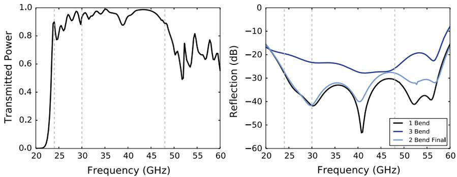
**Fig. 2** Left: the transmission of the OMT coupled to a feedhorn. Right: the reflection of the CPW-to-MS transition is shown for the 1 bend (black), 3 bend (dark blue), and final 2 bend (light blue) designs. The 2 bend reflection is similar to that of the 1 bend design, while the 3 bend design has significantly more reflection. The vertical dashed lines indicate the band edges (Color figure online)
