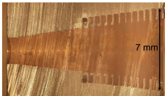
Figure 1: A cross section of the 90/150 GHz ACTPol feedhorn design is shown above. The first five corrugations on the left are ring-loaded. The dark spots in the bottom ring-loaded features are air bubbles in the wax filling the feedhorn, not defects. The pixel-to-pixel spacing on the AdvACT 90/150 GHz arrays is too small to allow for the corrugated feedhorn design.
